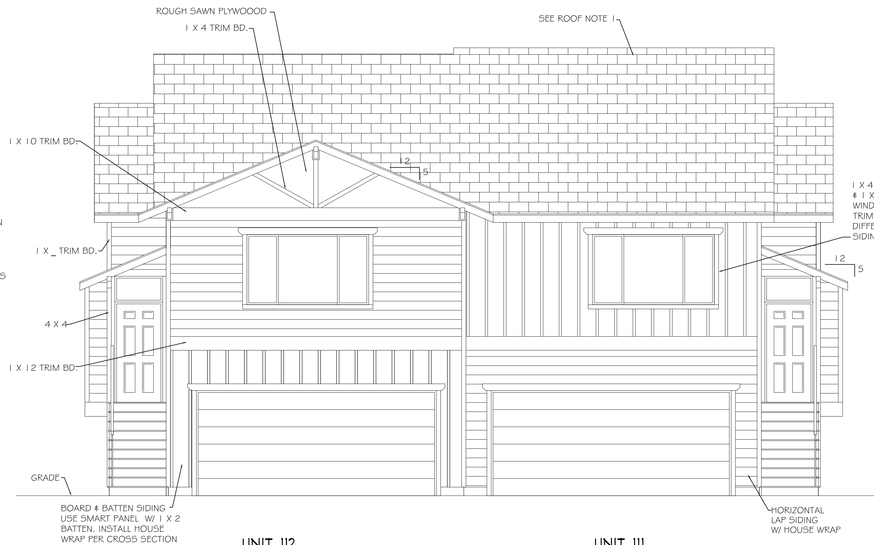
FRONT ELEVATION "B" SCALE: 1/4" = 1'-0"
